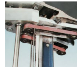
Automatic sharpening device with grinding belts
